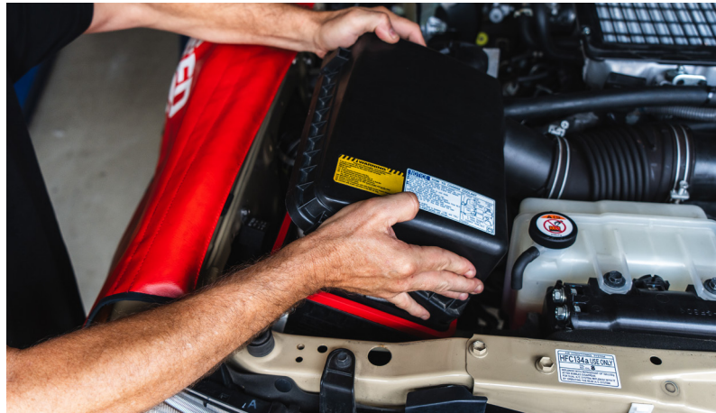
IMAGE 1 Filter removal from airbox.
