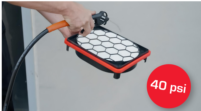
IMAGE 2 Clean out the dust trapped in the filter.
