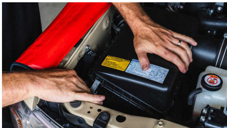
IMAGE 3 Put the filter back into the airbox the same as it was originally fitted.
