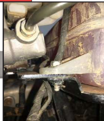
FIG. 10D CATCHCAN BRACKET INSTALLED
