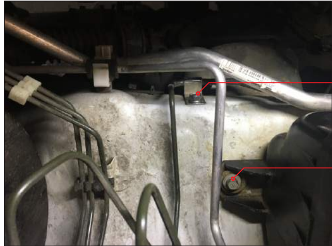
FIG. 13 AIR BOX BOLT REMOVAL
