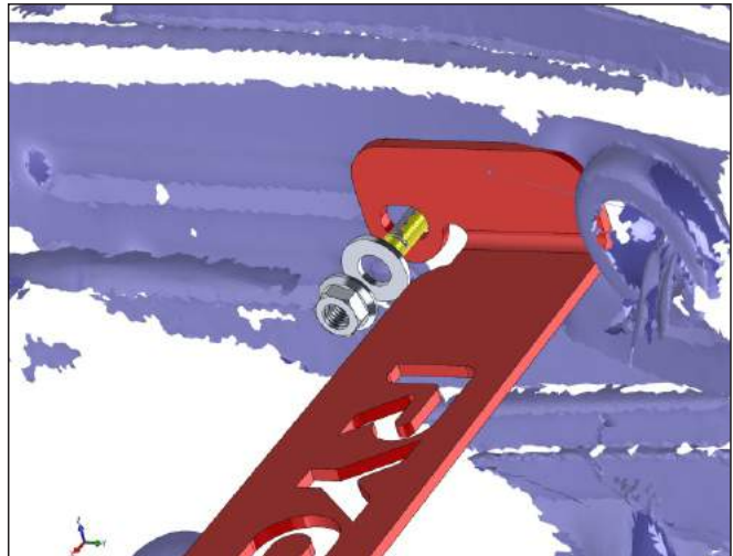
FIG. 19B BOLT AND WASHER FITMENT TO CATCHCAN BRACKET
