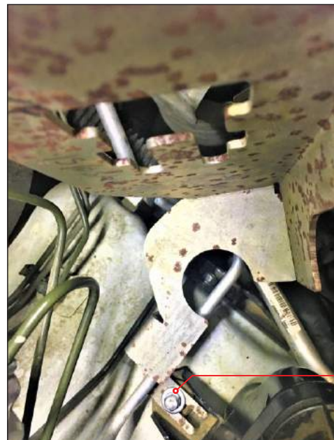
FIG. 18 RYCO AIR BOX BOLT & WASHERS FITTED
