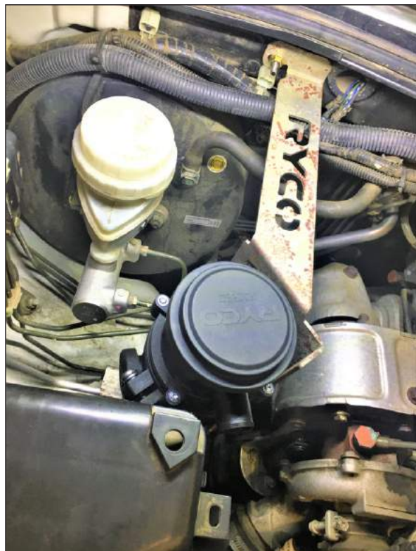
FIG. 20 CATCHCAN FITTED TO CATCHCAN BRACKET
