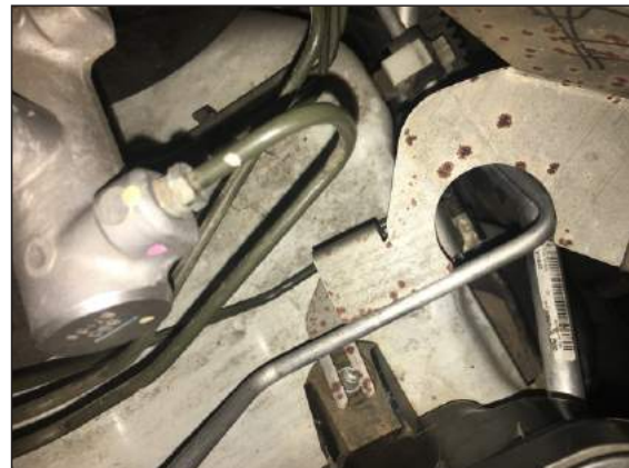
FIG. 17 FB9813CC FITMENT LOCATION, BEHIND AIR BOX VIEW
