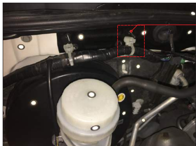
FIG. 15 PLASTIC CLIP REMOVED
