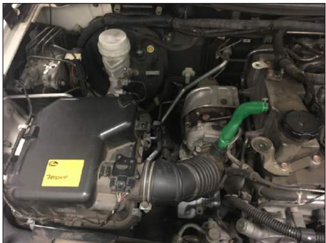
FIG.12 OEM PCV HOSE REMOVAL
