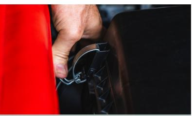
${\bf STEP~1}$  Start by undoing the clips on the intake airbox, lift the lid away and remove the old air filter.
