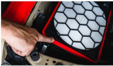
STEP 4 Check that the filter's seal is properly placed within the airbox.
