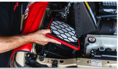
**STEP 3**Place the new Ryco NanoCel® Performance Air Filter inside. Make sure it is face (honeycomb structure) up.
